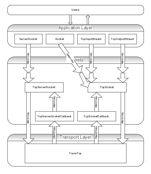
The following is a diagram of how they are connected:
