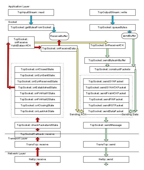
The arrows with red color indicates the execution flow when a packet is received. Then, in method onReceiveValidDataorACK in TcpSocket, it is divided into 2 paths. The first path is when data packet is received (still in red). The second path is when ACK is received, denoted by yellow arrows. From the diagram, it can be observed that after receiving data, the arrow becomes yellow since TCP will send acknowledgement packet after receiving data.
