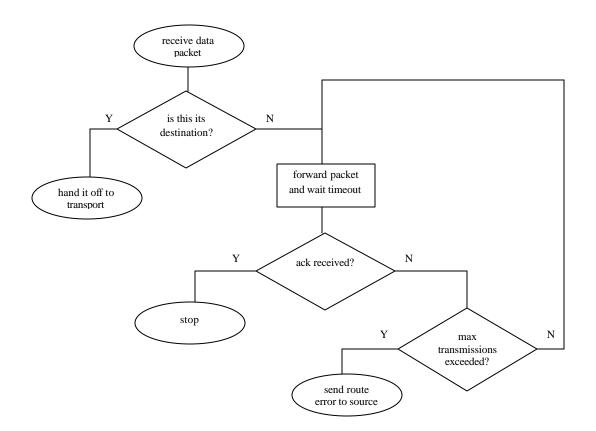
Figure 2 – Receipt of a data packet
